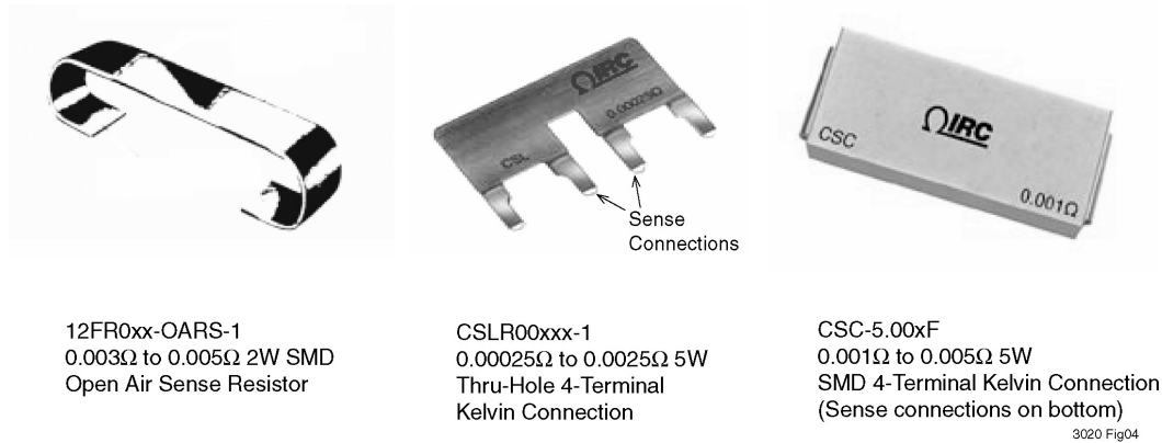
Figure 4. Current Sense Resistor Types.
