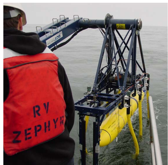
Figure 3. Deployment of the MBARI Mapping AUV using the AUV Launch and Recovery System (LRS) [17] on the R/V Zephyr.
