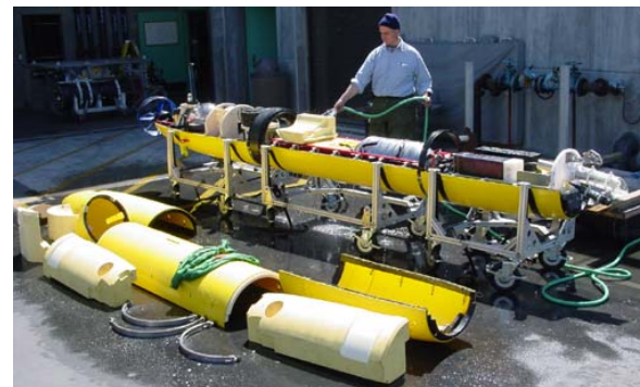
Figure 2. The interior of the MBARI Mapping AUV revealed by removing the upper fairings and syntactic foam blocks.
