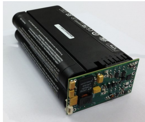
Figure 1 Battery Controller and two battery packs
