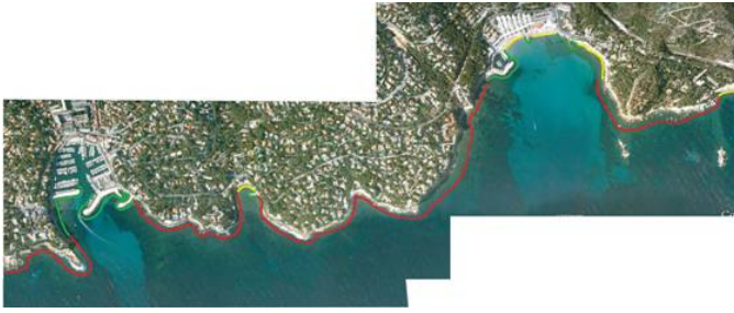
Fig. 4. Mobile laser scanning survey area – red lines represent cliff areas. Yellow lines represent beach areas. Port/harbor facilities (green) were not included in the study.
