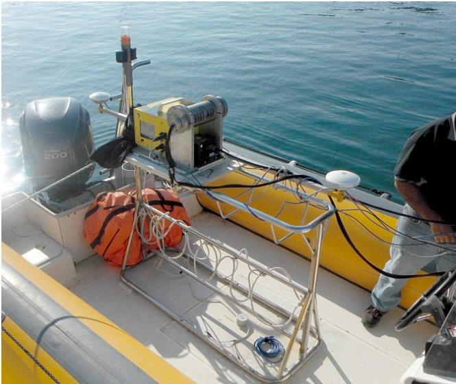
Fig. 5. Mobile laser scanning system (laser scanner, GNSS, IMU, and camera) installed in small vessel for survey.
