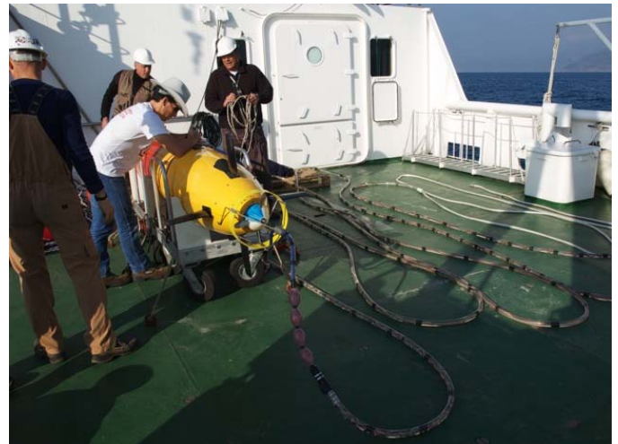
Fig. 3. BENS array attached to OEX-C AUV before its deployment at-sea from ALLIANCE
