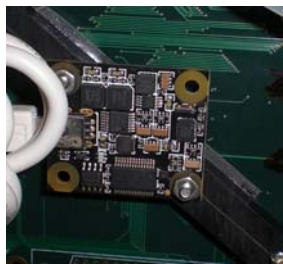
Fig. 11. Wave estimation payload. Full payload Hardware (top), IMU/Gyroscope/accelerometers/compass Phidget spatial 1056 sensor package (bottom)
