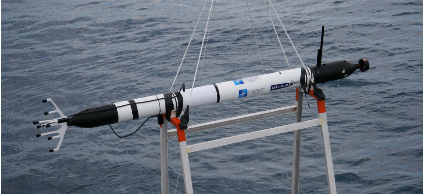
Fig. 7. eFolaga hybrid AUV/glider equipped with volumetric array payload. It is mounted on a bottom-moored frame for fixed position acoustic measurements
