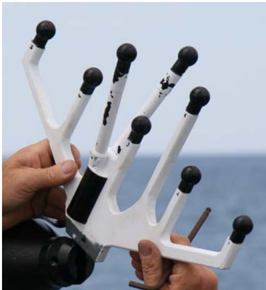
Fig. 8. Volumetric (tetrahedral and vertical) array of the eFolaga.
