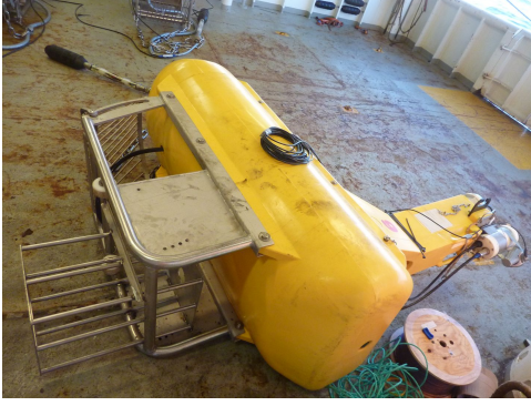
Fig. 1. Tailbuoy with underneath protective housing for USBL transceiver
