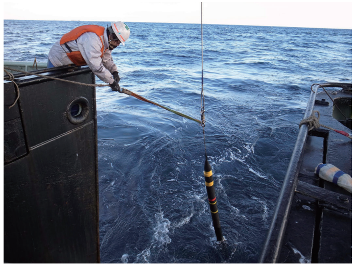
Fig. 6. Deployment of towed gamma ray spectrometer off Miyagi, Japan.
