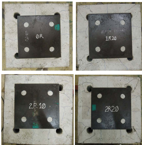
Fig. 7 Crack pattern of specimens
