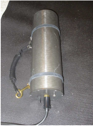
Fig. 2. The battery module is configurable for both cylinder-mount and side-mount options. This image shows the side-mount configuration with removable carrying handle, pressure-relief screw, and main power toggle switch.
