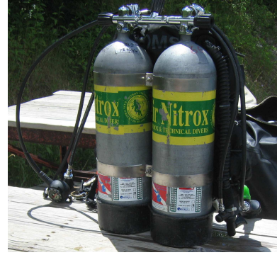
Fig. 1. Assembled technical rig with backplate, harness, wing, regulators, and double cylinders.
