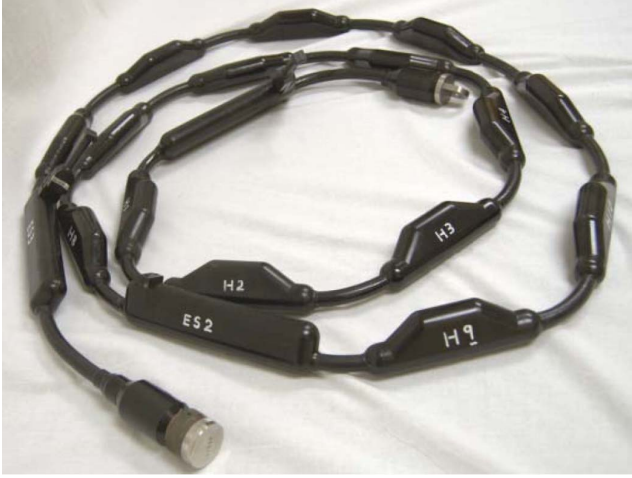
Figure 1. The multi-channel hydrophone array to be used with the Wave Glider.
