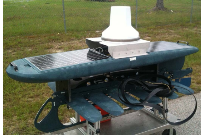
Figure 3. Wave Glider with integrated Satcom radome.
