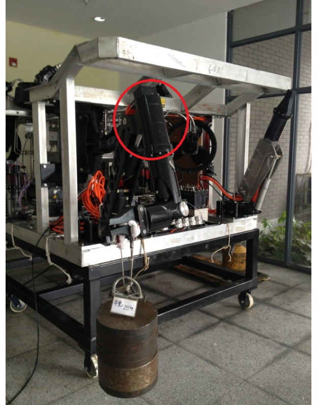
Fig.6. 7 function manipulator lifted a 100kg's weight
