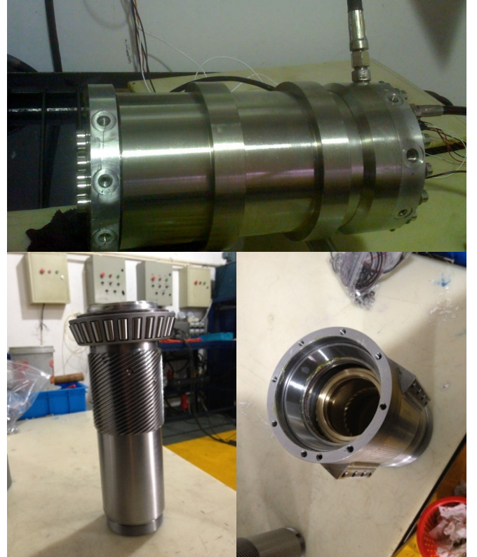
Fig.3. Hollow axis swing cylinder based on double screw pairs for manipulator's elbow joint, and its parts (shaft axis, cylinder, and piston etc.)
