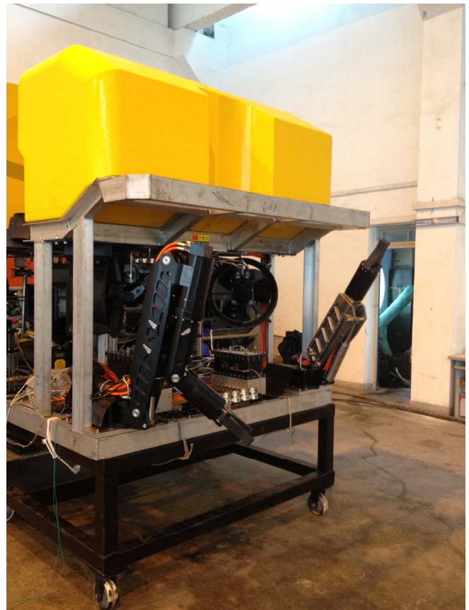
Fig.1. 7 function manipulator with a 270° rotary elbow joint
