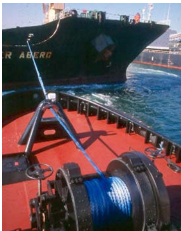
Fig. 1. Example of an application of a rope with Dyneema®: harbor towing on drum winch.
