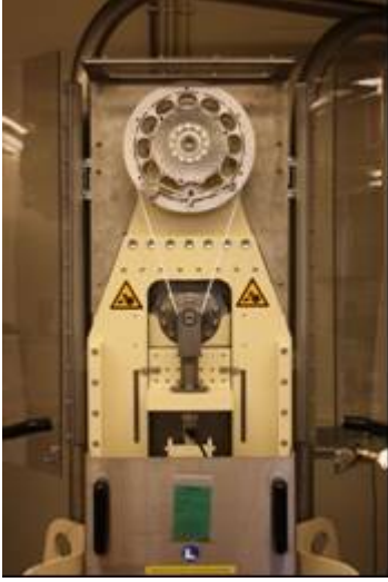
Fig. 3. Overview image of the bending over sheave test set-up.
