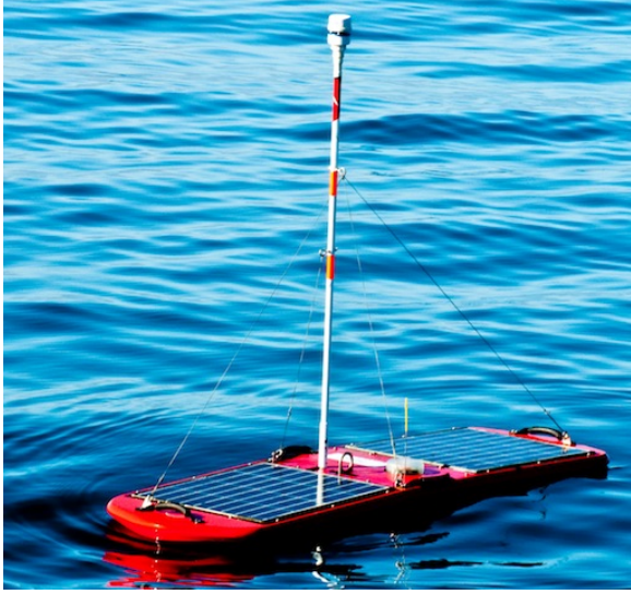
Fig. 2: The Liquid Robotics Wave Glider platform.
