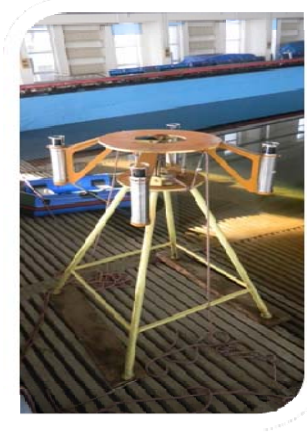
Fig. 6. Schematic of the responder array deployment in the AUV docking trial
