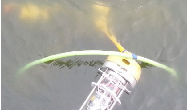
Fig. 14. AutoLARS homing on to an AUV
