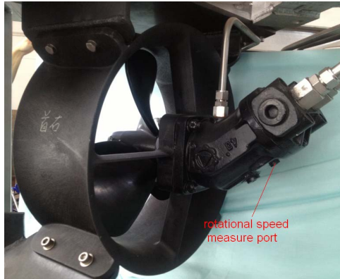
Figure.4. The 16" thruster installed on ROV
