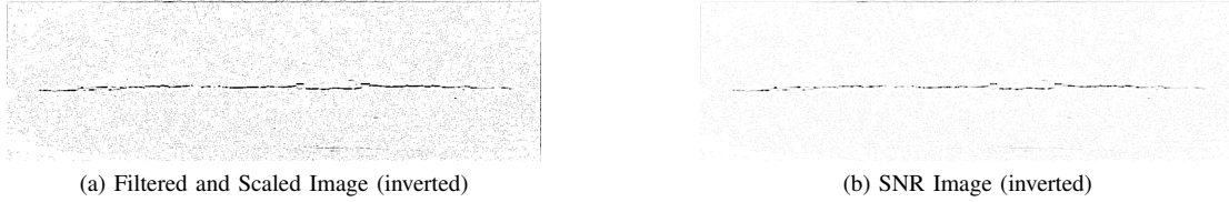
Fig. 2. Bandpass filtered image after the background was removed (figure 1b) and its corresponding signal to noise ratio.
