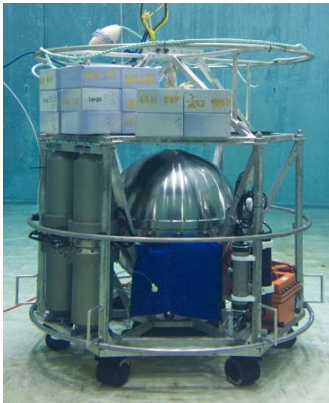
Fig. 2. Deep-ESP lander being tested in seawater tank prior to deployment. The titanium sphere houses the ESP instrument (center); the green towers are the DWSM (left); the dark bag in front of the sphere is the ambient oil reservoir (center bottom); the orange boxes are batteries (right); and syntactic foam blocks trim buoyancy (top).
