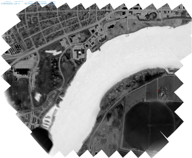
Figure 10: Mapped tiles are stitched together to form a mapped single image over the Columbia River. This nighttime image shows the Columbia River as it meanders, revealing the river surface structure. The pilot of the aircraft was instructed to follow the river. Here the control software was able to easily and successfully collect Mode 3 imagery over those aimpoints that fall within the sensor system field of regard.
