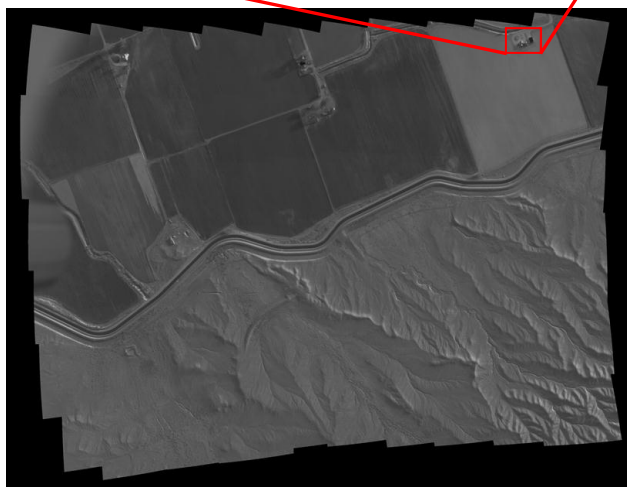
Figure 7: 60 image tiles are registered, mapped and stitched together to produce a single large image. A zoomed section of the image is expanded to reveal the details in the high-resolution imagery.
