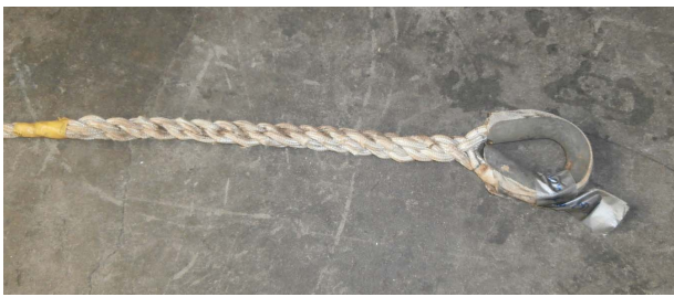
Figure 10. Original nylon mooring line eye.
