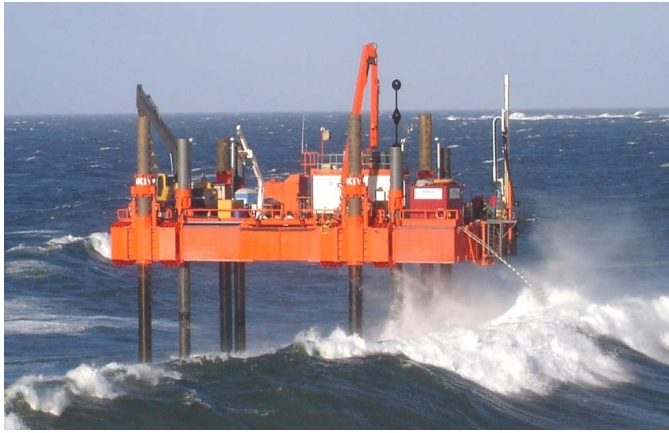
Fig. 6. Geotechnical drilling from offshore jack-up rig.
