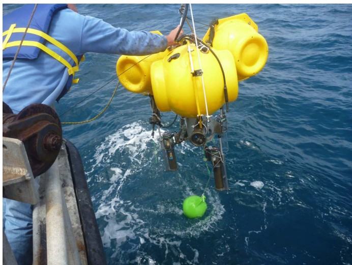
Figure 3: Recovery of MFC vehicle with full sediment tubes.
