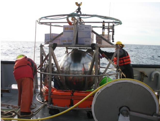
Fig. 11. The sphere, mounted in a freefall benthic lander, is being readied for deployment in the Monterey Canyon from the R/V Point Lobos.
