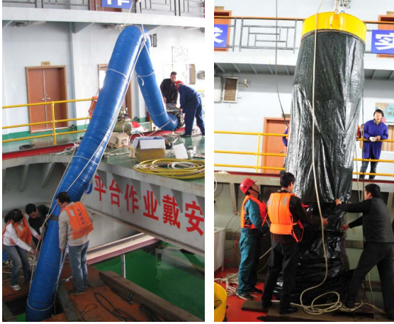
Fig. 2. Structures of the upwelling tubes: (a) the ventilation pipe directly applied; (b) the upwelling tube with inner support rings
