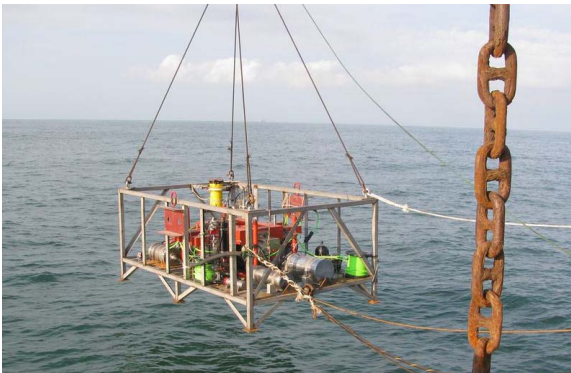
Fig. 6 Shallow sea test of the 10 kV powered system [20]
