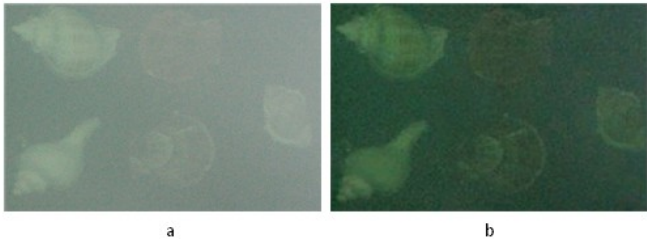
Fig. 9: The transparency is 70cm and the target distance is 1 time of visibility, the original image is shown in the left and the processed image is shown in the right.
