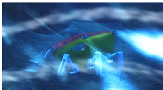
Fig. 2. Concept of overcoming strong tidal current by body posture control
