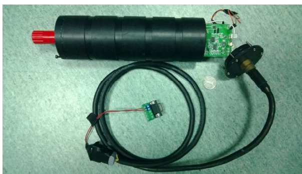
Fig. 2. The data logger inside the cylindrical pressure vessel (90 mm × 300 mm) with a water resistant connector
