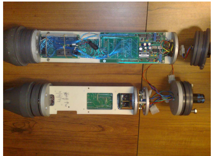
Fig. 2. The MAVS 1 (top) is a single board but with leaded parts. The need to incorporate RAM data logging with the TT4A controller when there was too little space necessitated interconnecting the RAM expansion board to the TT4A board with wire wrap wires in blue. By contrast the MAVS2 (below) with the same circuit but constructed with surface mount components contained the extended RAM without such extraordinary means. The compass and tilt sensors are at the right end of the chassis.
