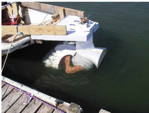
Figure 6 - PfISH turbine with backflow preventer and exhaust vanes, mounted for testing
