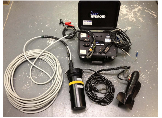
Figure 4. Towfish (TF) stand-alone modem
