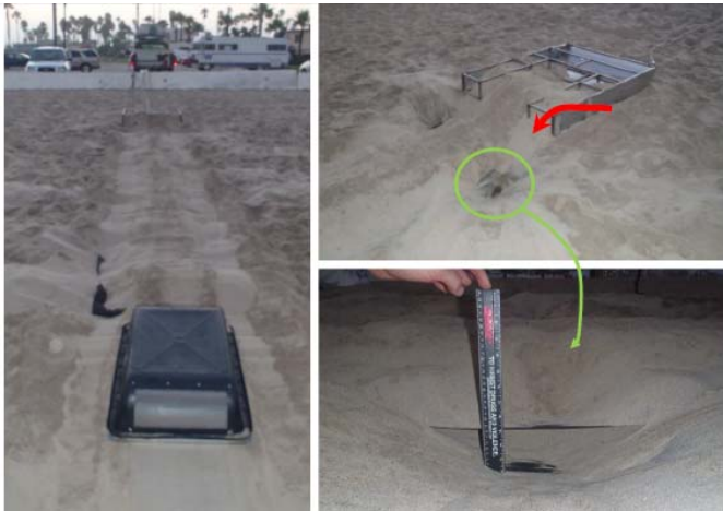
Fig. 8. Dry land testing of the double-blade sled. The arrow points to the two anodes.
