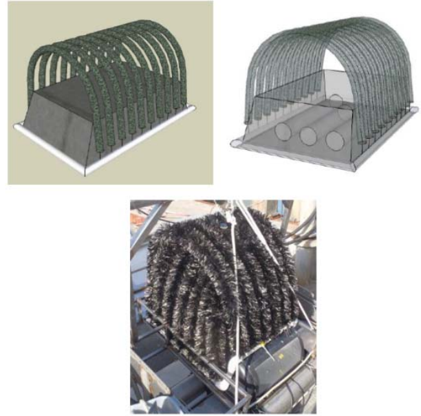
Fig. 5. New instrumentation pod with larger cathode carrying capacity.
