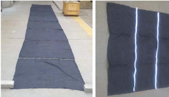
Fig. 3. From left to right 1. An array of anode modules 2. An anode module.
