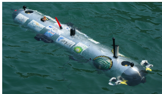
Fig. 1. The Autonomous Underwater Vehicle Nessie . On the front, a Tritech Gemini 720i is mounted.
