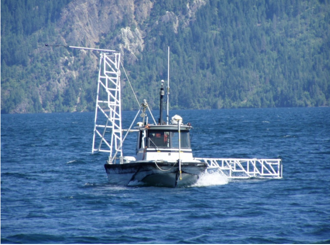
Fig. 4. The objective ship used during field testing. The MSBL transponders are attached to outriggers mounted on the sides of the ship, one of which is seen here raised to prepare for docking.
