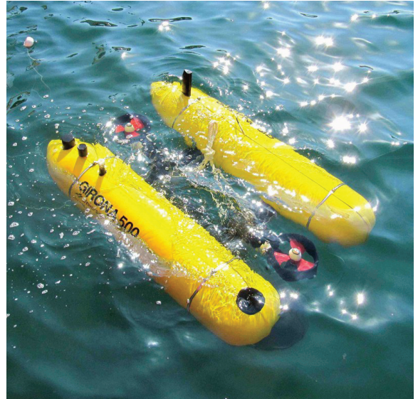
Fig. 1. The Girona 500 hover-capable AUV getting disturbed by waves in open water. A dynamic model of this AUV, obtained through system identification [8], is used for the simulated experiments described in this paper.
