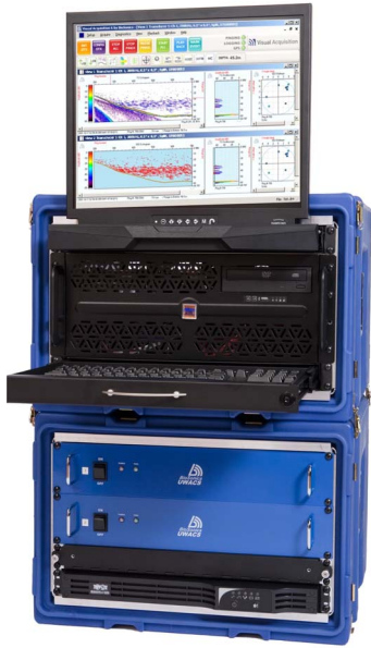
Fig. 2 Rack-mounted BioSonics DT-X Echosounder
