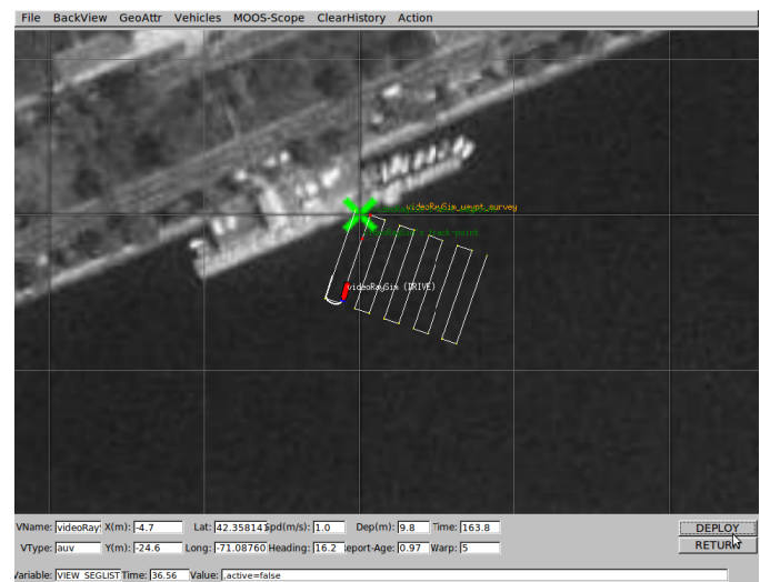
Fig. 2. The pMarineViewer application showing the UUV running the example search mission
