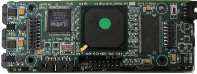
Fig. 5 - A photo of the WHOI Micro-modem showing the TI-6713 DSP floating point coprocessor board, which is required to receive PSK packets. The board set has a physical footprint of 4.5" x 1.75".
