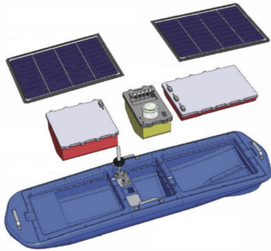
Fig. 3 - Engineering sketch showing Wave Glider float modules, including forward payload (left, red) where the REMUS Smart Gateway RF and controller electronics are integrated [4].
