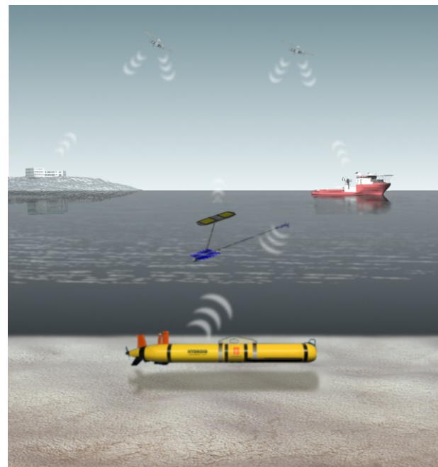
Fig. 1 – a rendering of the Concept of Operations for an ASV-hosted AUV communications and navigation aiding payload, showing Hydroid REMUS 600 AUV in acoustic communications with a Liquid Robotics Wave Glider SV2, which is acting as an acoustic-RF gateway, communicating via satellite to ship-based or shore-based operators.
