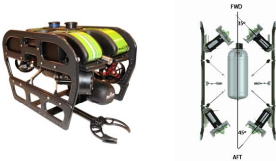
Fig. 1. The SeaBotix vLBV300 tethered AUV platform (left), and the planar vectored thruster configuration (right).
