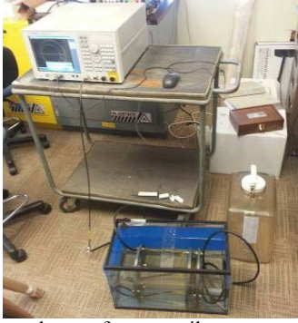
Figure 6. Experimental setup for two coil measurements in seawater.
