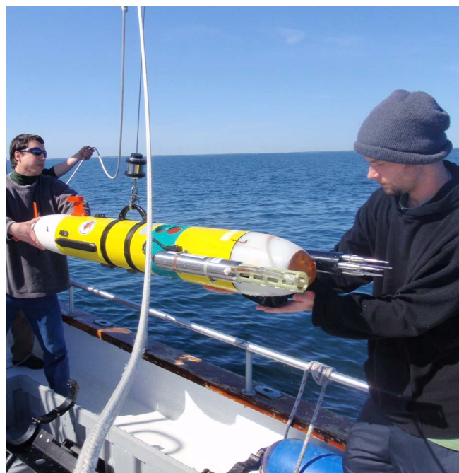
Fig. 1. The COAST PSM program provide opportunities for hands on experience with state-of-the-art technology. This autonomous underwater vehicle is equipped with a variety of sensors to measure ocean currents and turbulence (photo credit: Frank Smith)
