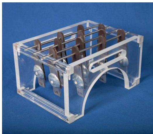
Fig. 2. A set of twelve individual peel samples hung by their tails from metal rods fitted into slots on top of the acrylic holder-racks, before immersion in a salt water test tank.
