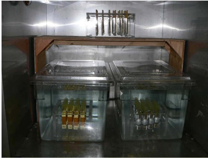
Fig. 3. Experimental set-up for peel samples and test racks maintained at elevated temperature. Samples in air are on top; samples in the salt solution without sacrificial anodes are in tank on the left, and samples in the salt solution with sacrificial anodes attached are in the tank on the right.
