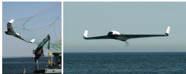
Fig. 3: X8 UAV used for the experiment. Landing (left) and fre-flying (right)
