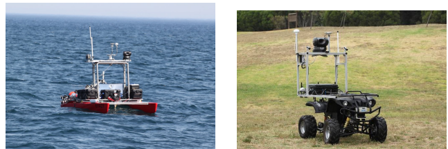
Fig. 1. Left: ROAZ II - Autonomous Surface Vehicle (ASV). Right: TIGRE - Autonomous Ground Robot for Outdoor Exploration
