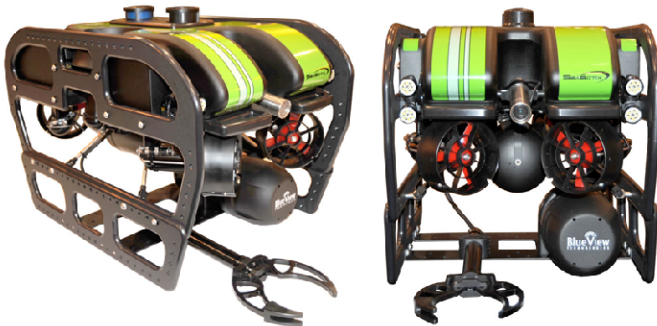
Fig. 1. SeaBotix vLBV300 miniROV platform ( www.seabotix.com ) has been modified to allow tethered, autonomous operations.
