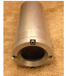
Fig. 4. Pressure housing showing planar lens with camera
