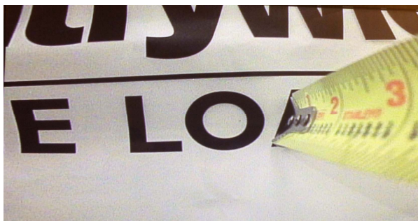
Fig. 5. Minimum focusing distance is 4.5in. Closest distance before black to white transition is no longer sharp.
