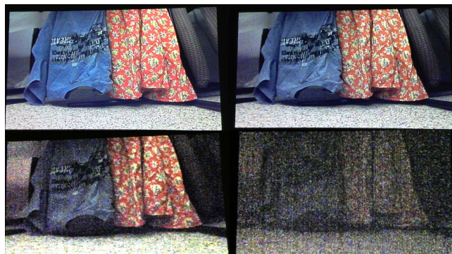
Fig. 6. Color mode performance. Top left: Full brightness at 36.2 Lux. Top right: Fading color at 11.5 Lux. Bottom left: Notable increase in noise at 1.15 Lux, Bottom Right: Image reduced to subject outlines at 0.27 Lux
