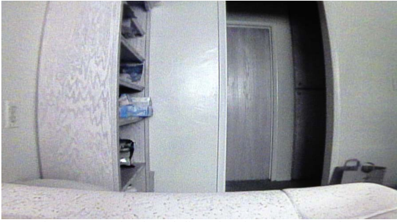
Fig. 8. Increasing barrel distortion from center to edges.
