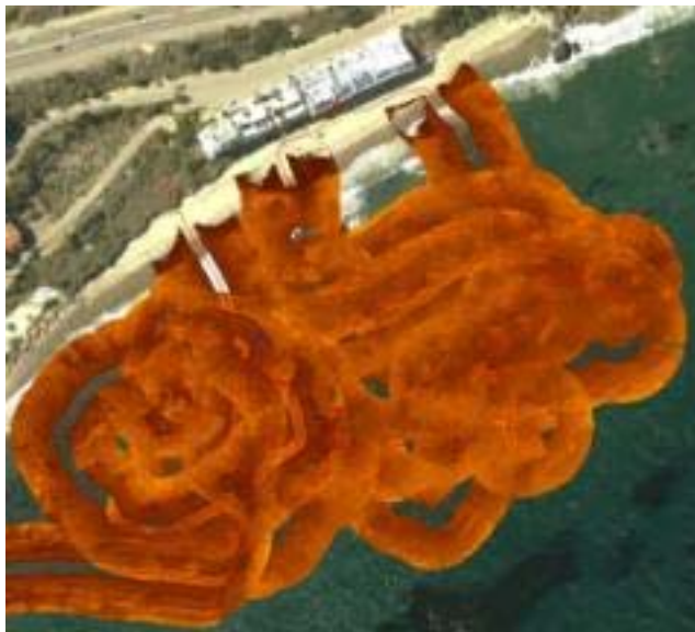
Fig. 6. Georeferenced side scan sonar map generated from a remotely operated Micro-USV searching for a sunken yacht. Malibu 2010. (Courtesy SeeByte)
