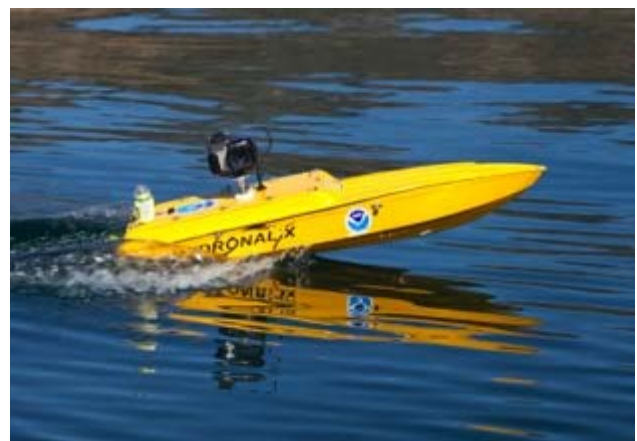
Fig.5. Micro-USV platform equipped with a high-resolution camera used by NOAA for imaging mammals and other animals in their natural habitat.
