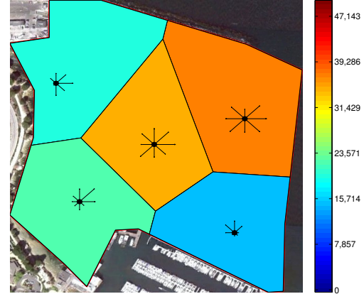
Fig. 8. The GCM created from the July 2012 data collection. The colors correspond to general assessments of signal strength and the vectors centered on the central cell node correspond to directional signal strength.
