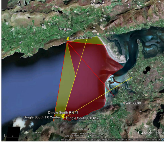
Figure 2. The map of the central part of Dingle Bay showing the 2 barrier headlands and the channel in between. The aerial photo (Google) shows the shallow bathymetry of channels and sandbanks. The geometrical overlays show the configuration of the radar stations. The southern station (St1) scans its beam about the yellow line at 57^\circ E; and the northern station (St2) scans between the red lines. The area common to St1 and St2 is that which may produce current vectors; shown as maroon in the schematic.
