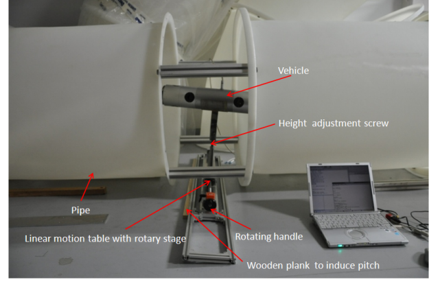
Fig. 9. Ground truth image capturing setup
